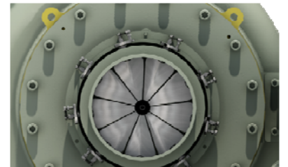
Figure 2: Front-view of IGV in fully-closed position.
