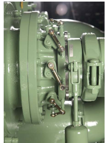
Figure 3: Side-view of mounted IGV showing the yoke assembly and actuator.
